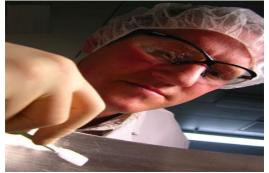
Swab accuracy determines a method's ability to recover the compound of interest directly from the swab head.
